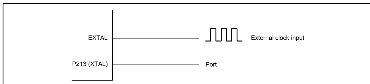
Figure 9.8 Equivalent circuit for external clock
