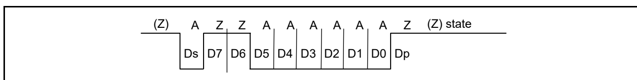
Figure 34.48 Inverse convention with SDIR in SCMR = 1, SINV in SCMR = 1, and PM in SMR_SMCI = 1
