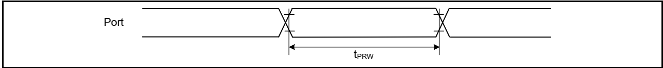
Figure 2.27 I/O ports input timing
